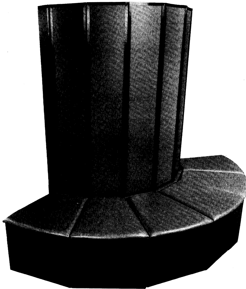
Figure 1-4. CRAY X-MP Model 22 or 24 6-column mainframe chassis
