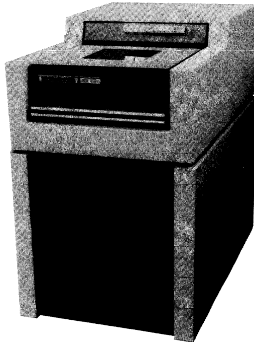
Figure 1-7. DD-29 Disk Storage Unit
